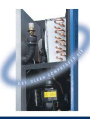
All GENESIS compressors are fitted with a built in air treatment package comprising refrigerant dryer with R134A gas, pre-filter, final-filter and modular condensate drain. The operation of the dryer and condensate drains is conveniently controlled by the compressors main MC2 controller this provides for efficient dew point control and allows the fridge compressor to cycle efficiently.
