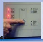
Press the Start button to start the welding process. The device will set the welding time automatically.
