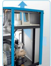
For installations that do not have continuous water cooling supply, the air cooled WIS® 40-75 series integrates air/air and air/water stainless steel heat exchangers. The footprint remains extremely low (2.35m²) compared to any external cooling device, and installation costs are reduced compared to the addition of external roof coolers. Coolers can be cleaned regularly by simply removing of the side panel. Cooling air outlet is located on the roof for easy ducting.
