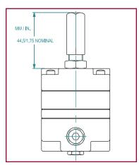
The Type 10 Regulator is available with a tamper-resistant cover, as illustrated. The cover is threaded over the adjusting screw to prevent inadvertent or unwarranted adjustment of output pressure.
