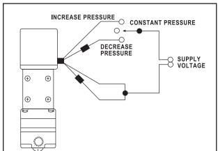
NOTE: To increase output pressure, apply voltage to unmarked leads. To decrease output pressure, apply voltage to marked leads.
