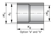
Option "a" - for rear mounting Option "b" - for front mounting
