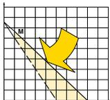
Theoretically torque curve change caused by throttling
