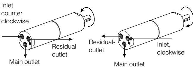
The direction of rotation of reversible motors is controlled by supplying inlet L or inlet R with compressed air. Air motors can be stopped and started continually without damage.
