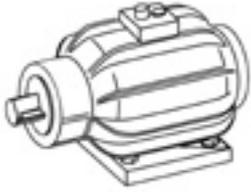
Air motors have much smaller installation dimensions than corresponding electric motors.
