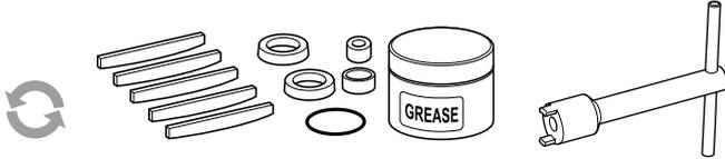
The first service is due after approximately 500 hours of operation. After the first service, the service interval is determined by the degree of vane wear. The table below shows new dimensions.
