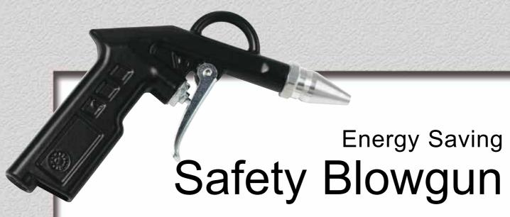
Energy Saving Safety Blowguns from Meech Air Technology combine an ergonomic lightweight gun handle with the Meech Nozzle (see page 6). Meech blowguns typically save up to 70% of compressed air usage compared to conventional types of blowgun whilst dramatically reducing noise levels.
