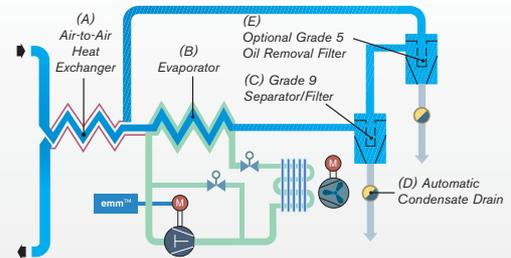
Figure 2 - Digital Evaporator Refrigeration Control
