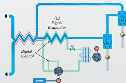
Figure 3 - Hot Gas Bypass Valve Refrigeration Control
