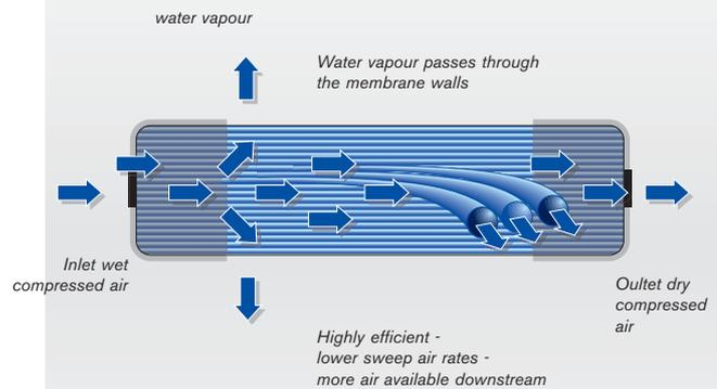
*The pressure dew point is influenced - among other conditions - by the size of the membrane surface and the time the air stays in contact with it. The longer air contacts the surface and the larger this surface actually is, the bigger the decrease of the dew point. Other conditions influencing the dew point are inlet temperature, inlet pressure dew point.*
