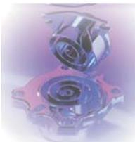
These innovative refrigeration scroll compressors are capable of running loaded or unloaded. Digital Scroll compressors unload by allowing the fixed upper scroll to move axially from the orbiting lower scroll.
