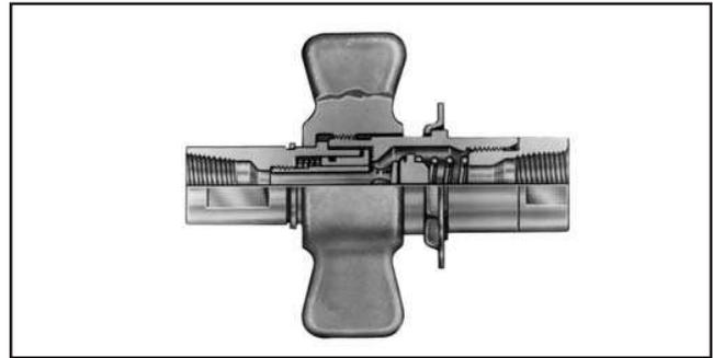
The 5100 Series brass coupling with steel tubular valve offers minimum air inclusion and fluid loss. Thread together latch provides connect under pressure capability and vibration resistance. It is not rated for continuous hydraulic impulse applications. (See FD86 on page 69.)
