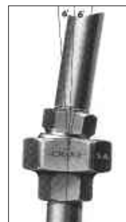
6° out of alignment and still pressure tight
