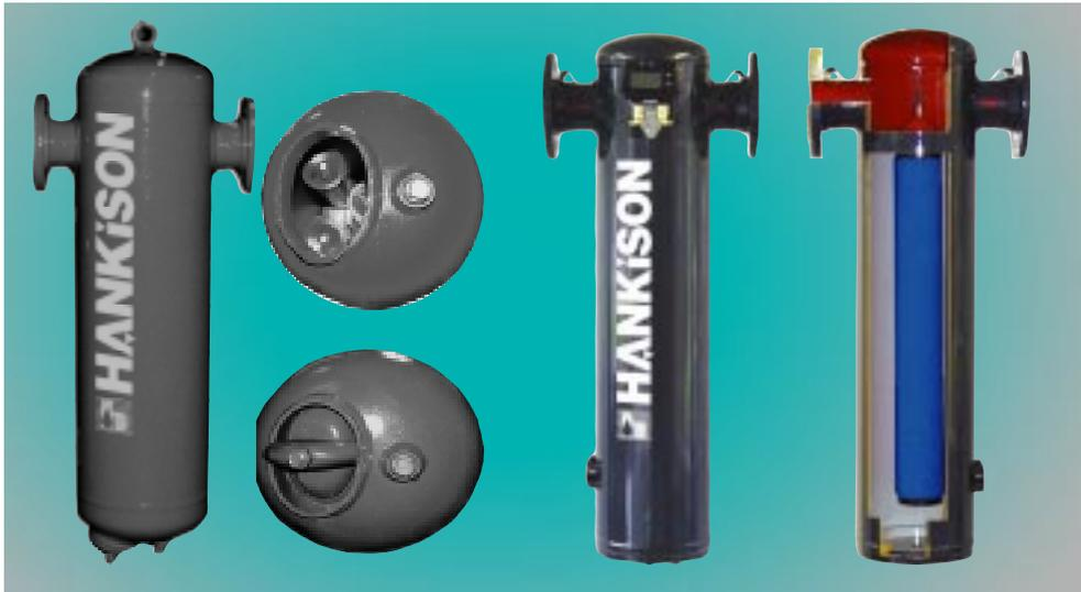
Filter sizes from HF-54 and larger are available with two different vessels. The standard filter vessels are equipped with a large handhole which can be opened with only one screw in order to change the filter elements.
